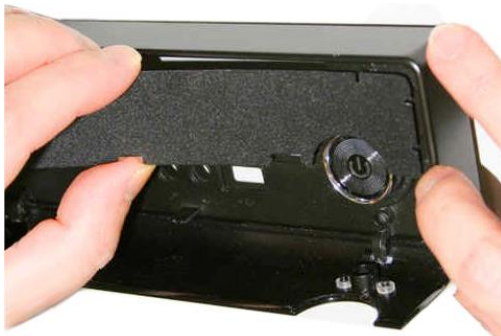
Installation of the self-adhesive mylar
