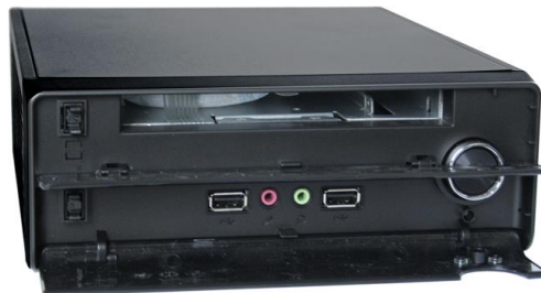
The PC with open front doors. The ODD bay remains empty.
